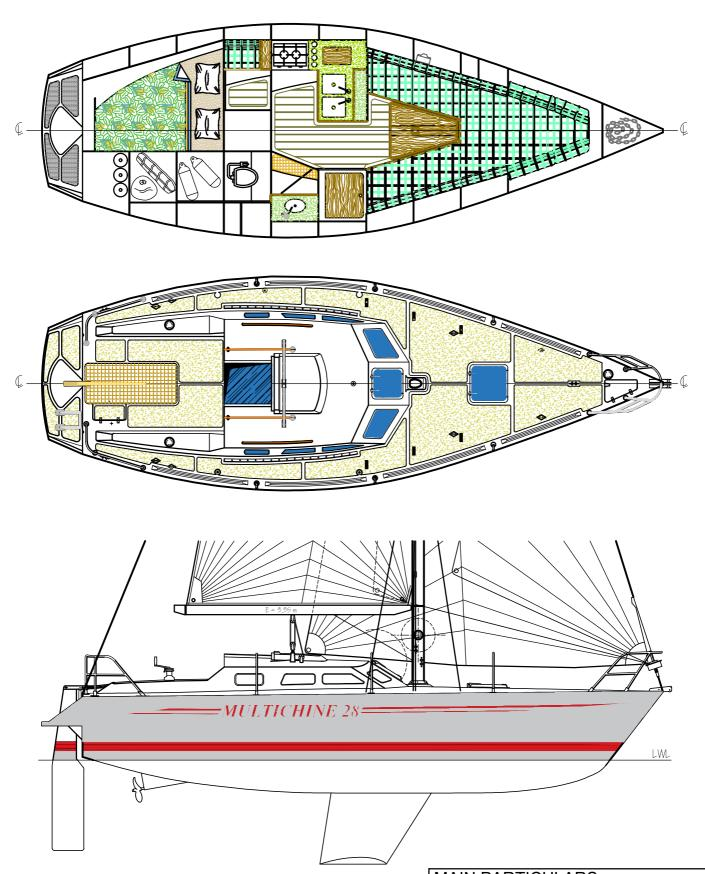
Construction: Wood/Epoxy - Plyglass
